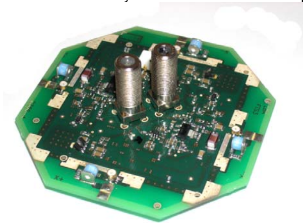
Figure 16. LBA active baluns pcb, RF shield has been removed.
