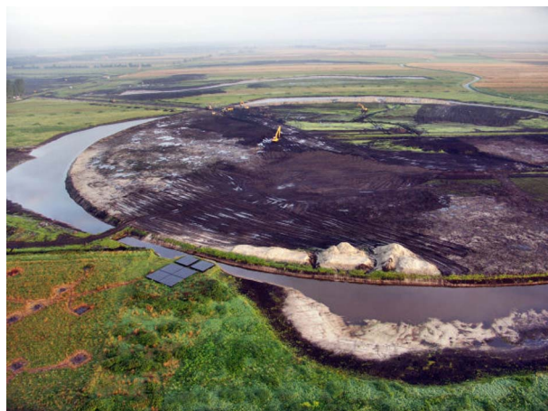
Fig. 6. The central area of the LOFAR core near the village of Exloo in The Netherlands. The inner circle has a diameter of 350 m and the total core area is approximately 2 km in diameter. In the lower left corner, part of a test station is visible. The black rectangles are HBA tiles. Some LBAs are only visible from the lack of vegetation around their groundplanes.
